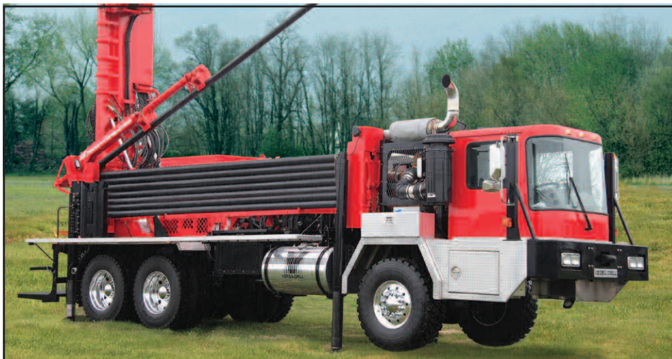
Versa-Drill's (patented) automated drill rod handling system; stores, handles and positions 500' of on-board drill rod.
