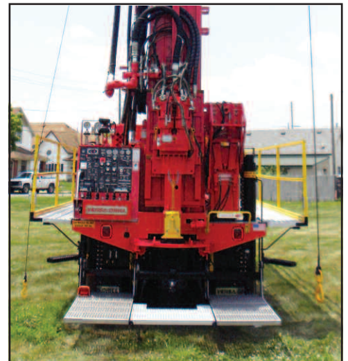
Operator-friendly control panel and hydraulic retractable split centralizer table.
