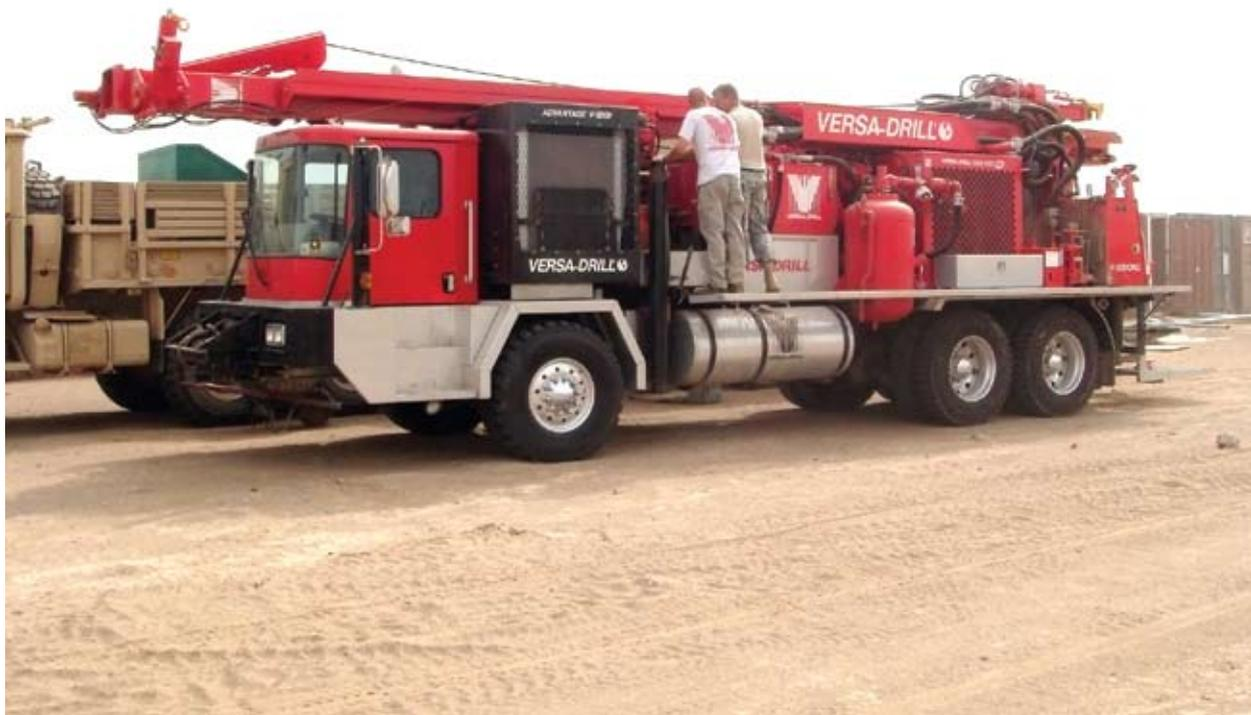
The Versa-Drill V-2000NG is inspected prior to field operation.
