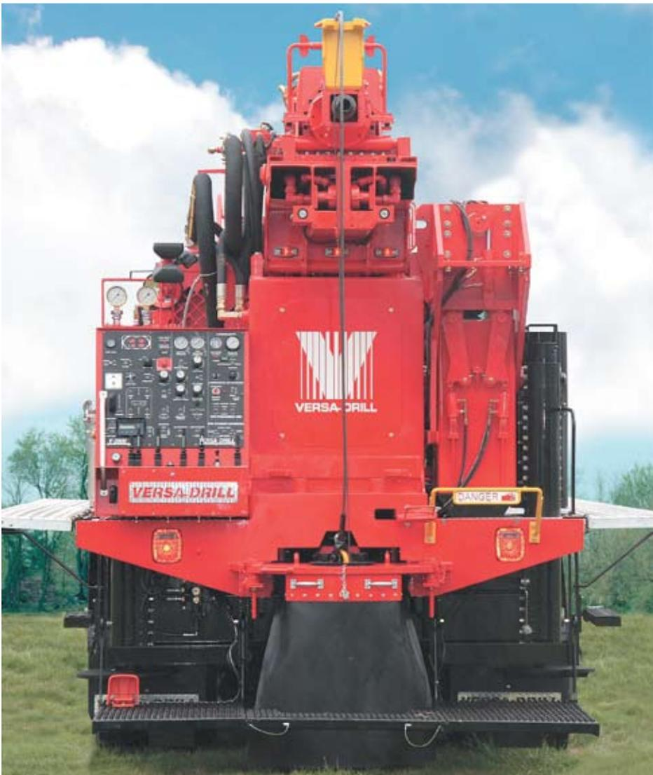
User-friendly electro/hydraulic controls with functionally grouped gauges and twin fold-up aluminum platforms.
